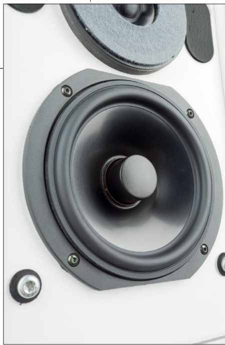
On the smaller of the two mid-range drivers, you unfortunately cannot see the dual-basket design from the outside
